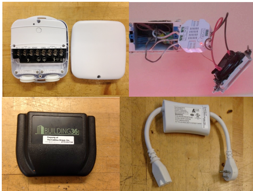
Figure 4. Technologies used (clockwise from top left: 220-volt z-wave energy switch, lighting wall switch, z-wave gateway device, and 110-volt z-wave energy switch). Source: Cadmus 2016
