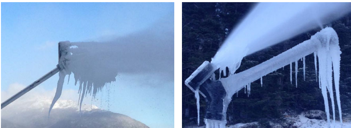
Figure 2. Unexpelled water creates ice build-up and reduces the efficacy of early energy-efficient snow guns. Source: VEIC 2014.
