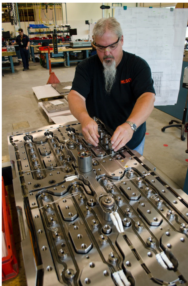
Figure1. Manifolds are manufactured from steel plates.
