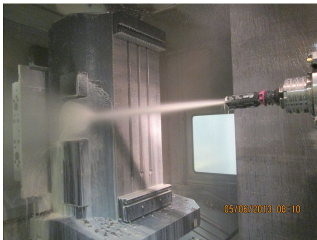
Figure 1. High-pressure metal cutter in operation.
