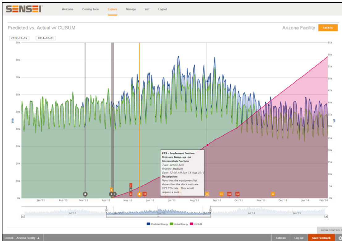
Figure 1. Sample EMIS chart showing energy model results overlaid with completed action items.
