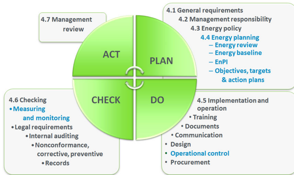
Figure 1. Mapping ISO 50001 elements to PDCA continual improvement (used with permission from the Georgia Institute of Technology [Georgia Tech]).
