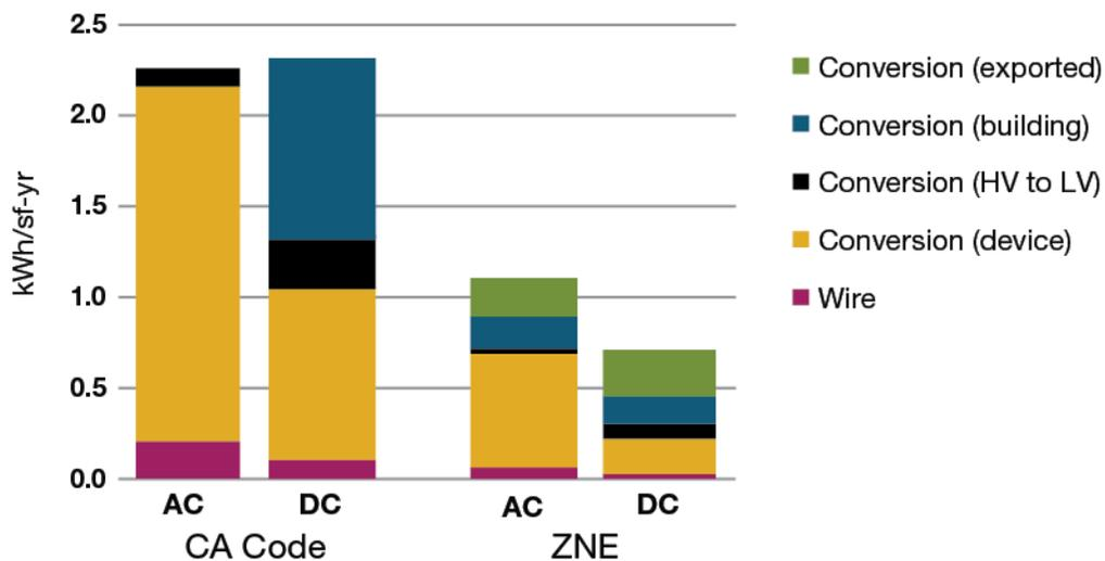
Figure 4. Estimated electric distribution and conversion losses in commercial office buildings.
