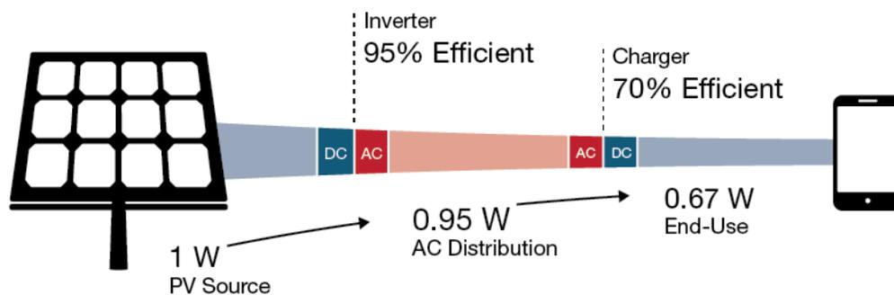
Figure 5. Conversion of 1 W from a PV panel (left) delivers 0.67 W of usable to an electronic end-use (right).
