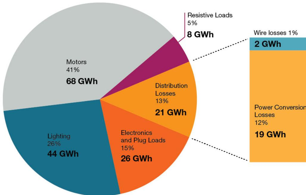
Figure 1. Loads and losses in California commercial office buildings (Ecova 2012).
