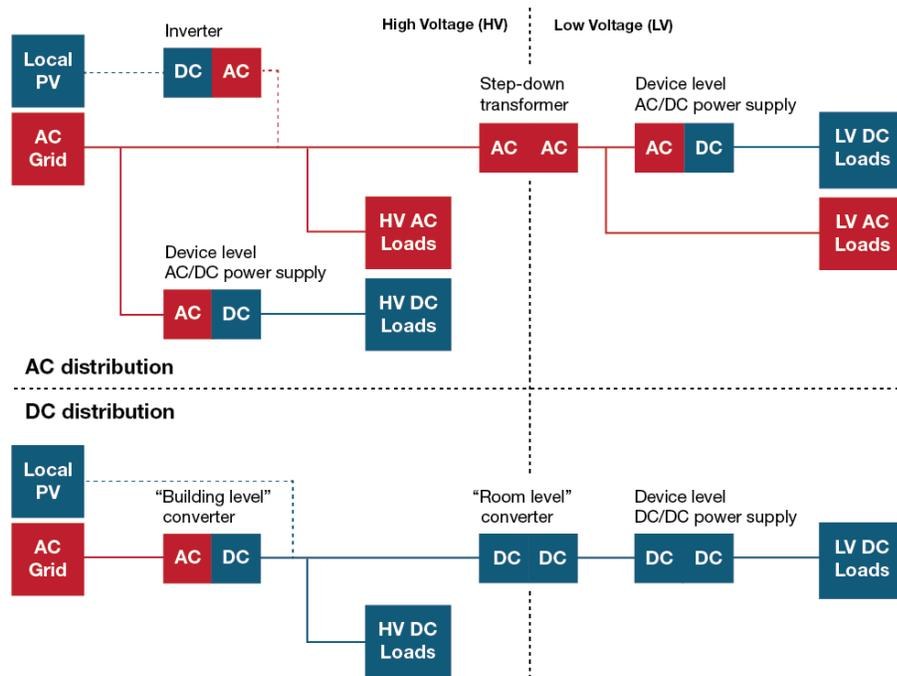
Figure 2. Schematic of AC and DC distribution approaches<sup>3</sup>.
