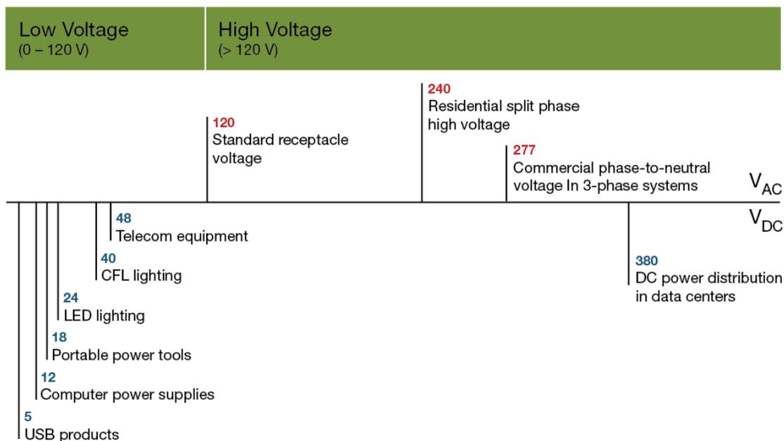
Figure 3. Common AC and DC voltages in high- and low-voltage products.
