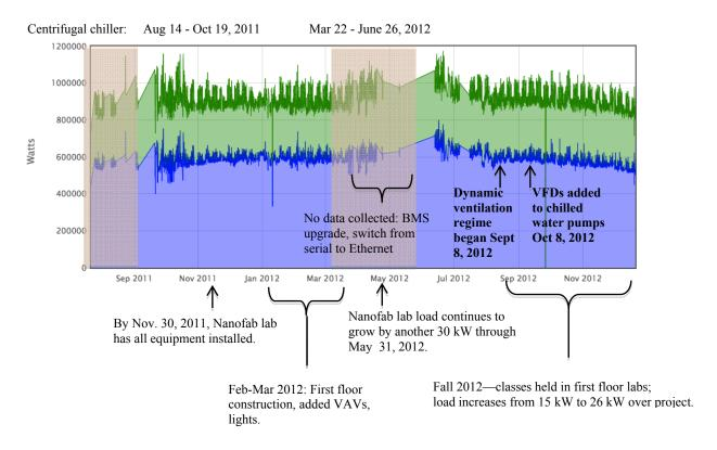
Figure 3. Whole building electrical load of Sutardja Dai Hall from May 22, 2011 to Dec 31, 2012 (MSA upper/green, MSB lower/blue) *Source*: Peffer 2012.
