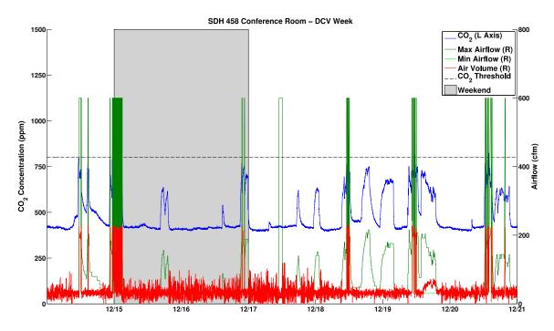
Figure 7. Operation of a conference room ventilation system with a demand-controlled ventilation strategy. *Source*: Taneja, 2013.
