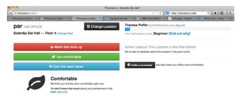
Figure 6. Web-based occupant thermal comfort control interface.
