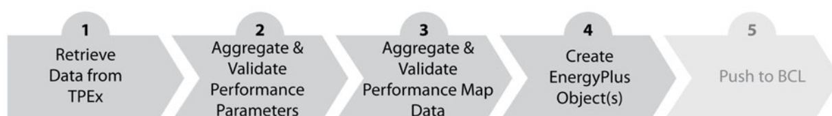
Figure 4. Overview of the process used to convert product-specific foundational energy performance data from the TPEX to EnergyPlus syntax. Source: Marjorie Schott, NREL.
