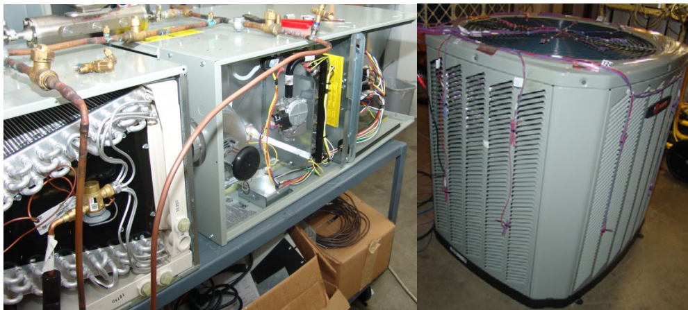
Figure 1. HVAC test unit - indoor unit (left), outdoor condensing unit (right).
