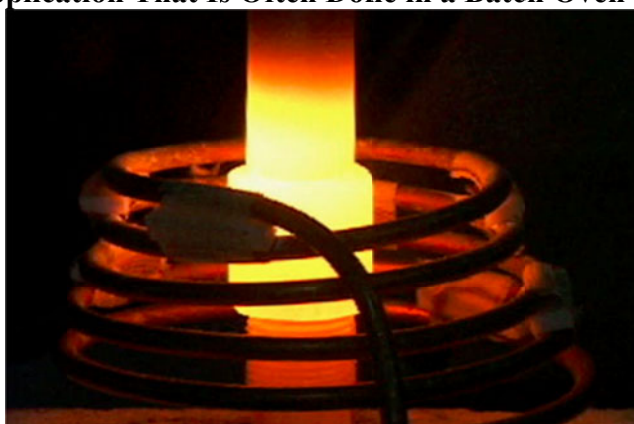
Figure 1. Copper Brazing of High-Pressure Steel Fitting Using Induction Heating— an Application That Is Often Done in a Batch Oven
