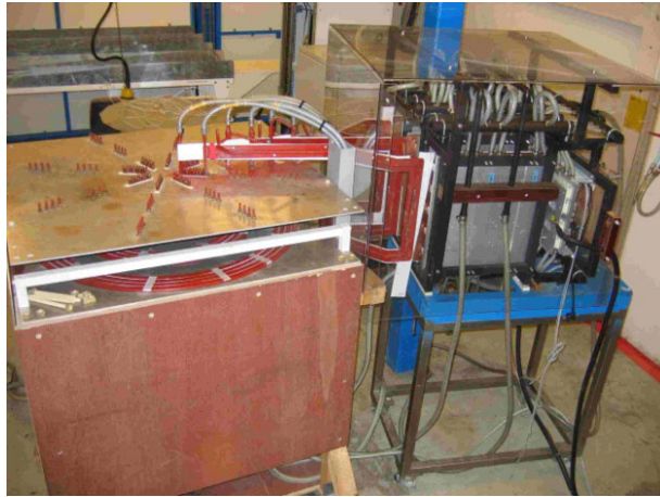
Figure 3. Model of Multi-coil Power Supply and Inductors with Three Associated Coils
