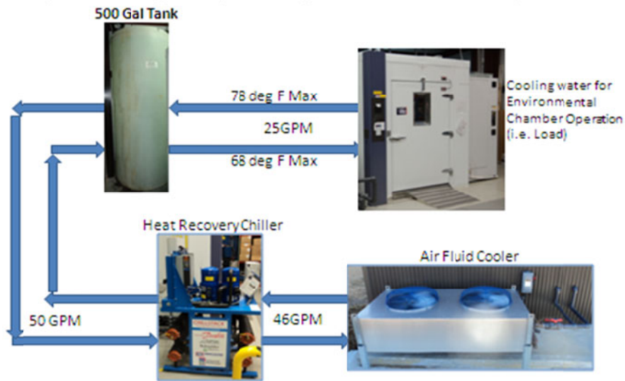
Figure 3. Simple Layout Diagram of Heat Recovery Chiller
