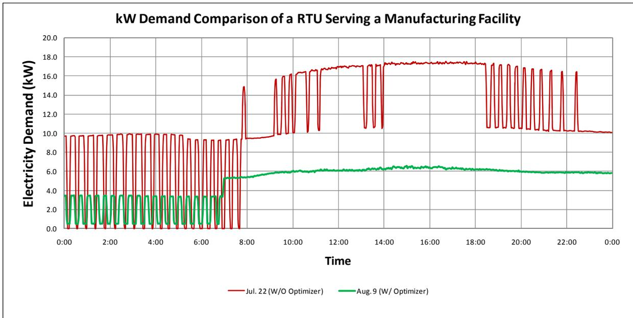
Figure 4 compares the daily kWh consumption of the two hottest days before and after the optimizer installation. The daily electricity consumption was reduced to 116.48 kWh from the before electricity consumption of 278.34 kWh. This represents a 58% reduction.
