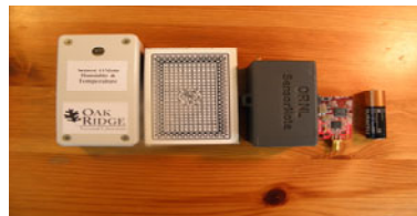
Figure 7. Prototypes of Inexpensive, High Performance Wireless Sensors Developed in the ITO-BTP Effort
