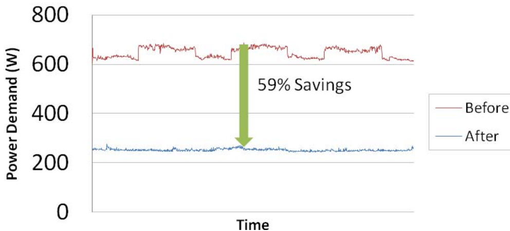
Rumsey Server Closet Power Demand Before and After Virtualization
