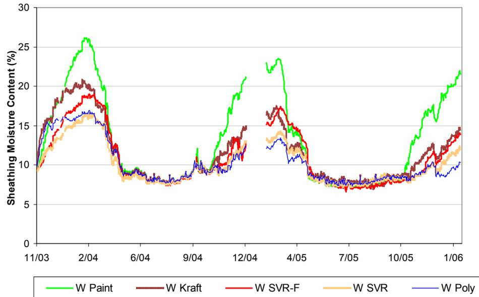
The latex paint walls clearly have the highest moisture contents, with peaks in the 20-25+% MC range; the south walls act similarly and are not graphed here due to space constraints. The remaining walls exhibit drier behavior, rarely rising above 20% MC; a typical threshold given for mold growth on wood is roughly 20% MC for several weeks. During the summer, all walls dry to very safe moisture content levels (less than 10% MC); it is difficult to distinguish between them during this period.
