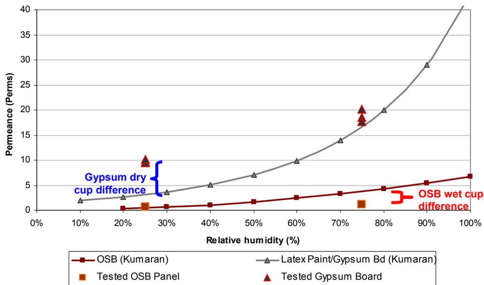
The test results at wet cup conditions for painted gypsum board are similar to published data. However, at dry cup conditions—closer to the wintertime operating conditions—the tested permeance is much higher, averaging 9.8 perms (compared to 3.1 perms in the literature). Although the tested specimen would meet requirements for a Class III vapor retarder, it was much higher than expected.
