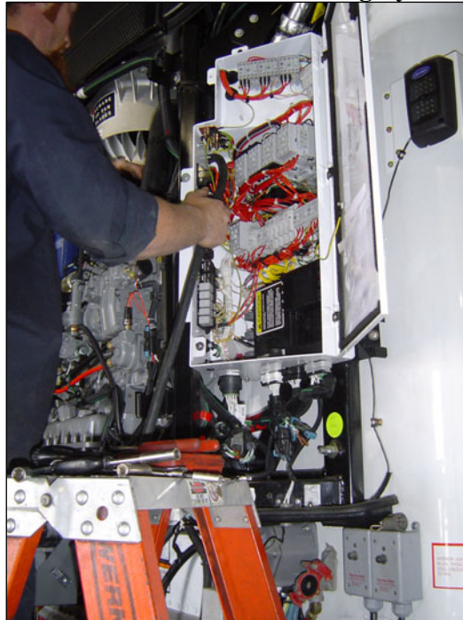
Figure 2. Connection of Trailer Wiring System to eTRU
