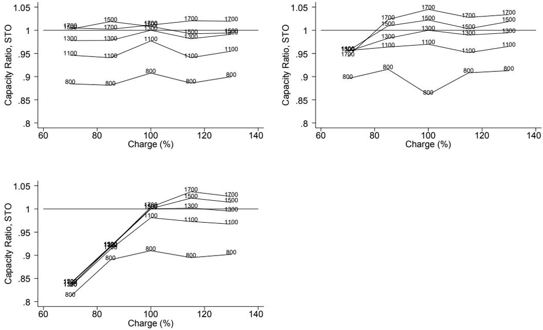
**Figure 2. Capacity Ratio (TXV) versus Charge at 3 Outdoor Temperatures**
