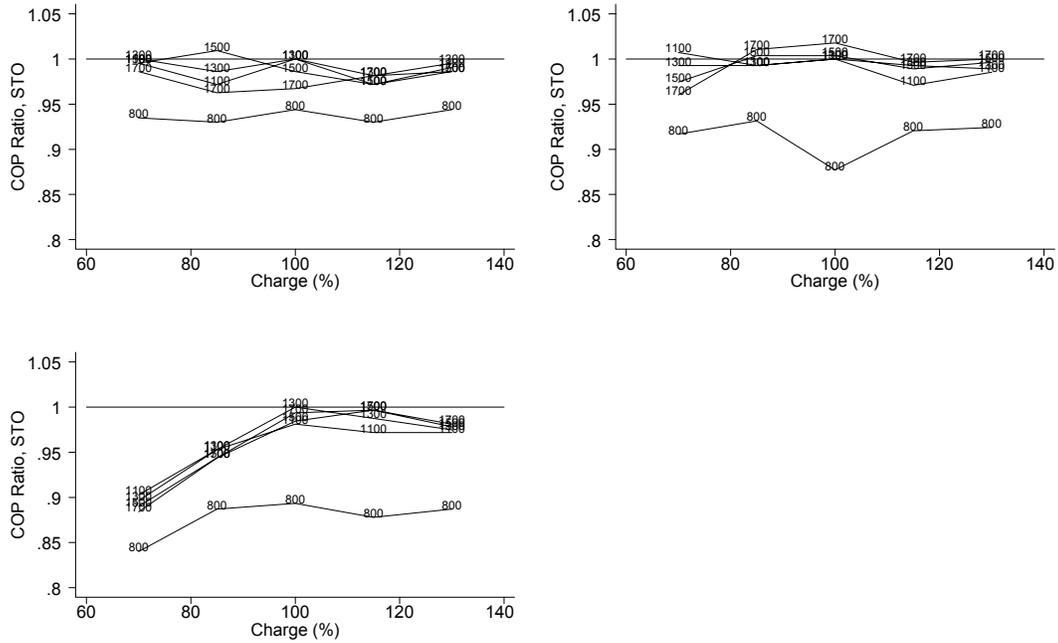
**Figure 4. COP Ratio (TXV) versus Charge at 3 Outdoor Temperatures**
