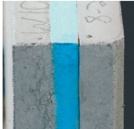
Figure 2. Cross Section of the Dow Chemical T-Mass™ Walls Used on the ZEH
