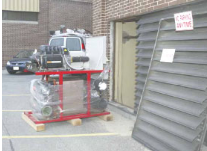
Figure 6. Multistack Turbocor Unit
