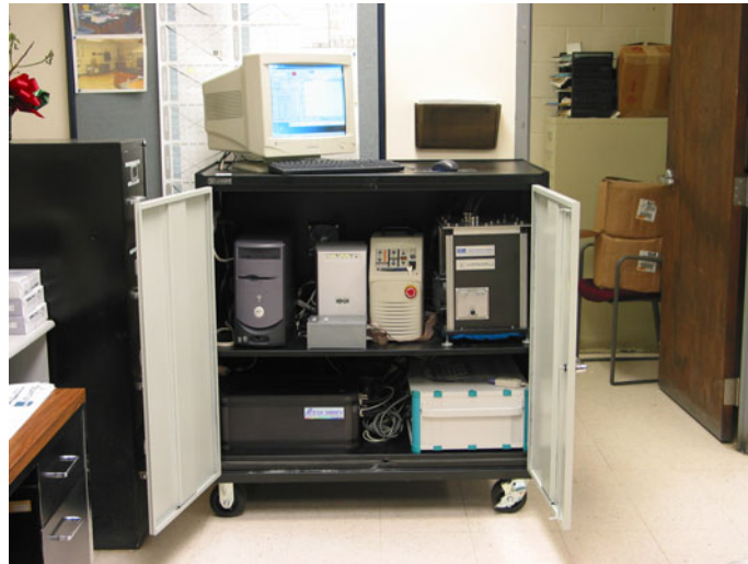
Figure 7: Photograph of ERCo Batch Analyzer Equipment in PPG Chester Plant
