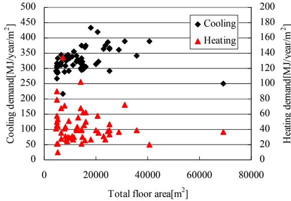
**Figure 13. Cooling and Heating Demand of the Saving Demand**
