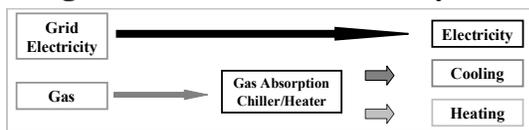
**Figure 7. Schematic of Individual CHP System**
