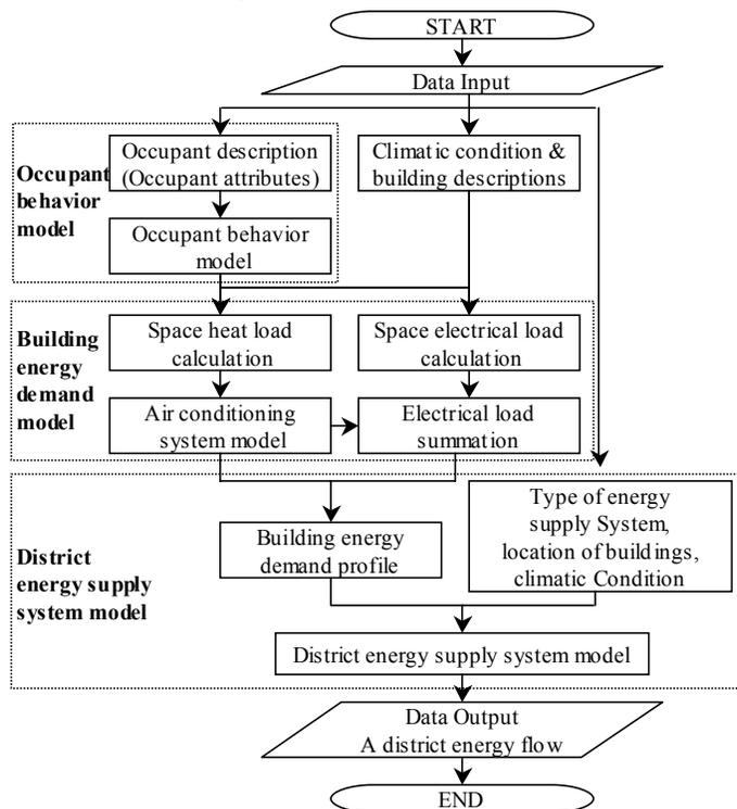
**Figure 4. Flow Chart of the Occupant Behavior Model**
