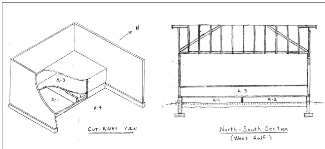
**Figure 2. Schematic of Test Space Layout**
