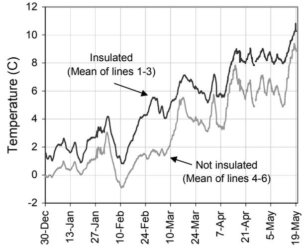
**Figure 7. Temperature History of the Foundation Exterior Surface**
