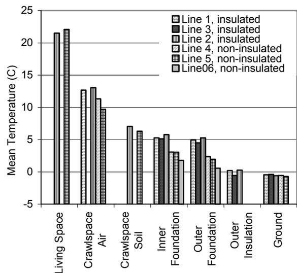
Figure 9. Temperature Profile through the System, February 27
