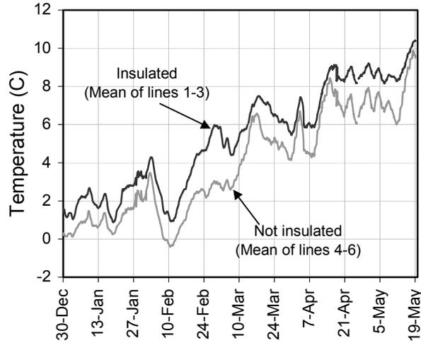
**Figure 6. Temperature History of the Foundation Interior Surface**
