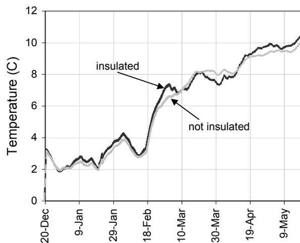
Figure 8. Crawlspace Soil Temperature History at 18in. Depth
