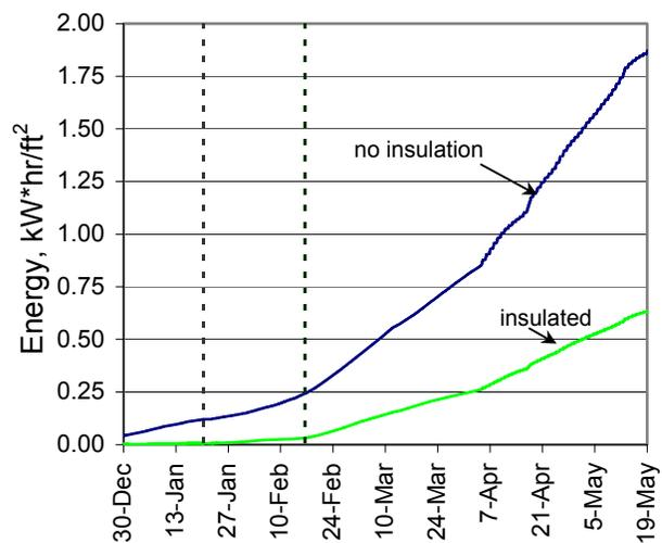
**Figure 11. Cumulative Energy Flow Through Foundation, per Square Foot of Foundation Surface**
