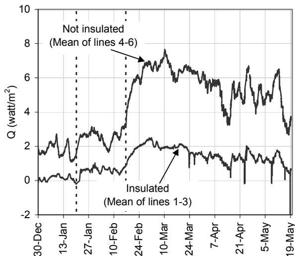
**Figure 10. Seasonal Heat Flux Through the Foundation Wall**
