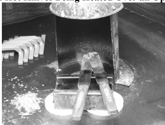
Figure 5. Hot Knives Being Heated Over an Open Flame
