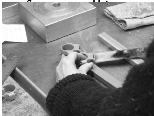
Figure 4. Worker Using Hot Knife to Apply a Wax Pattern to a Runner
