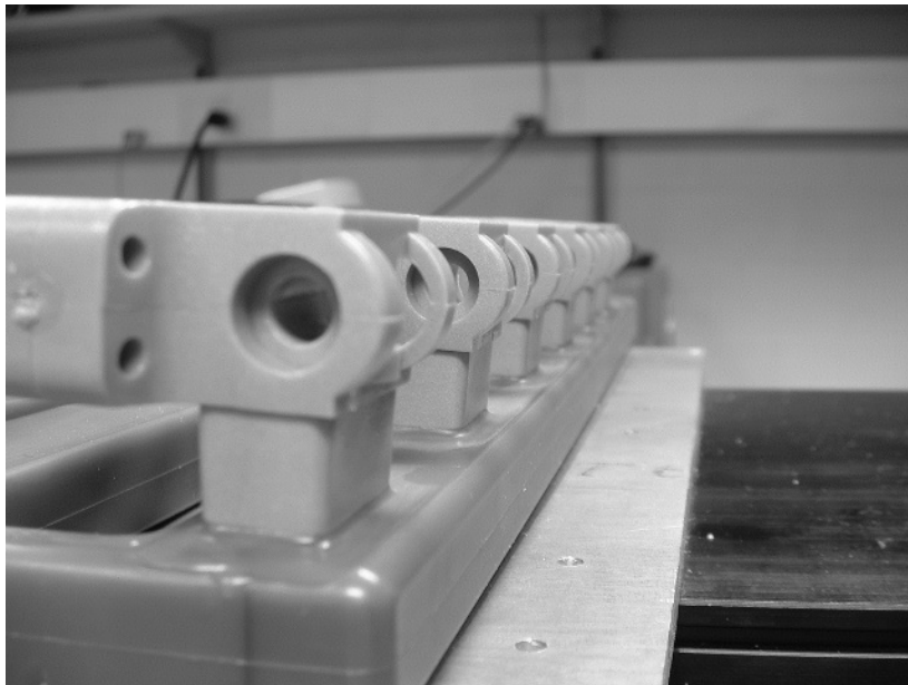
Figure 10. Populated Runner Showing Precise Alignment of Patterns
