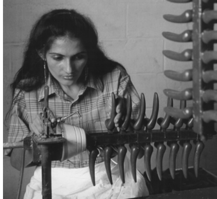
Figure 6. Worker Using "Sticky Wax" and Gas Torch to Apply Patterns to Runner
