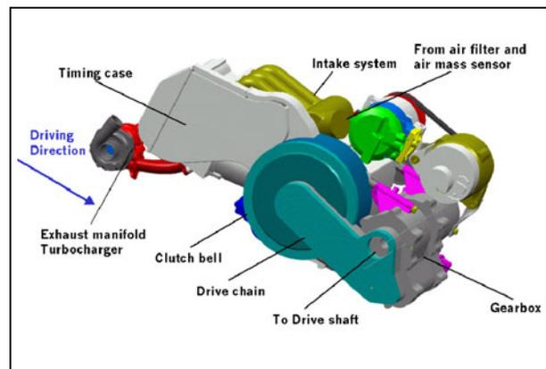
One of the most important contributors to fuel economy is the powertrain. The affordability target of the program eliminated the consideration of hybrid systems, such as internal combustion engines or fuel cells combined with an electric motor. The system had to meet the requirements of package space, affordability, torque and power, CO<sub>2</sub>, and mass. Calculations predicted that a conventional 1.2L gasoline or diesel engine combined with a
