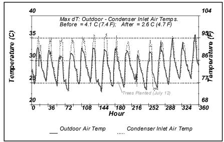
Figure 5. Plot of Long-Term Temperature and Insulation Profiles Before and after Landscaping at Site 1
