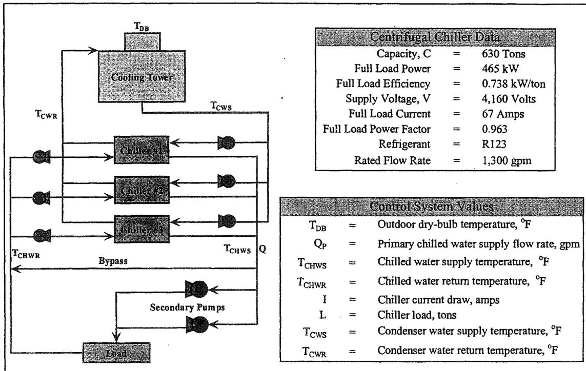
Figure 1. Chilled Water System Schematic, Chiller Data, and Control System Values
