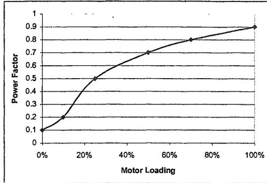
Figure 2. Power Factor Versus Motor Loading
