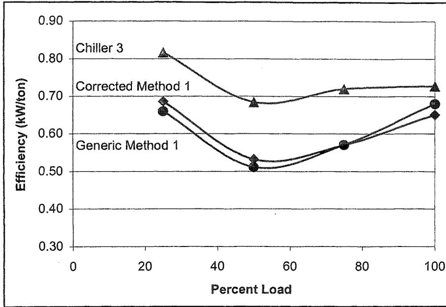
**Figure 4. Chiller Data Versus Method 1 Tool Data (Generic and Corrected)**
