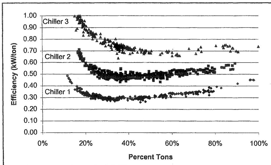
Figure 3. Chiller Performance Curves From System Data
