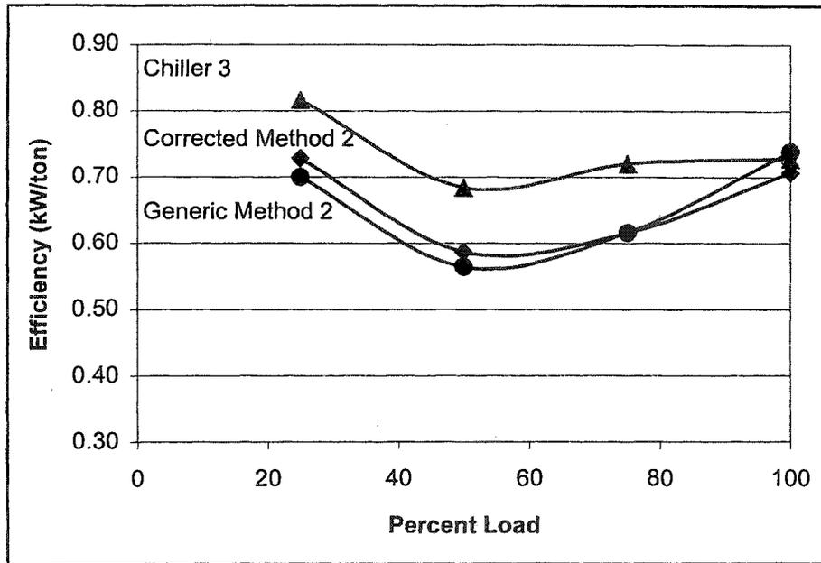
Figure 5. Chiller Data Versus Method 2 Tool Data (Generic and Corrected)
