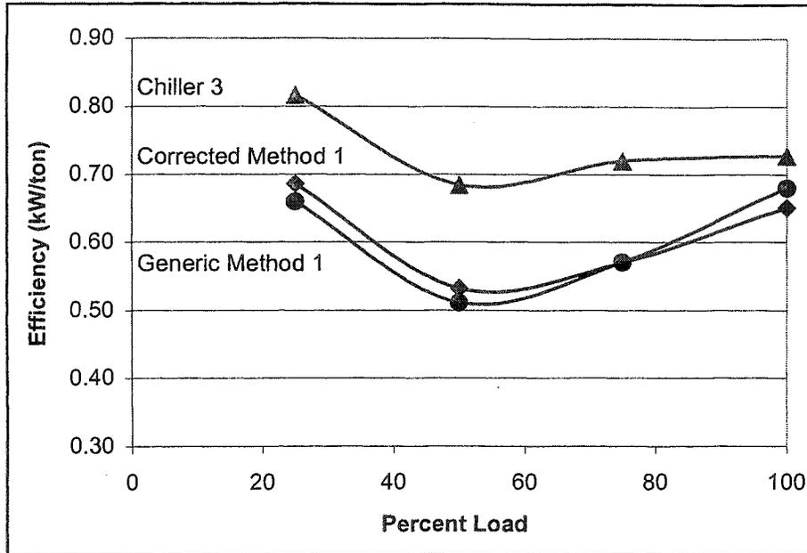
**Figure 4. Chiller Data Versus Method 1 Tool Data (Generic and Corrected)**
