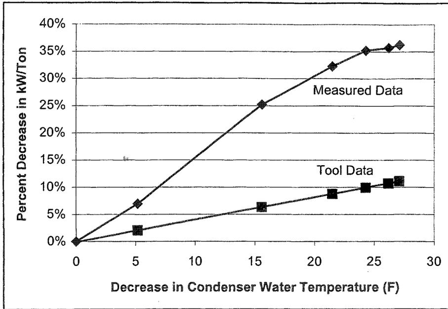
Figure 6. Effect Of Decreasing Condenser Water Temperature: Measured Versus Tool Data (Monger 1999)
