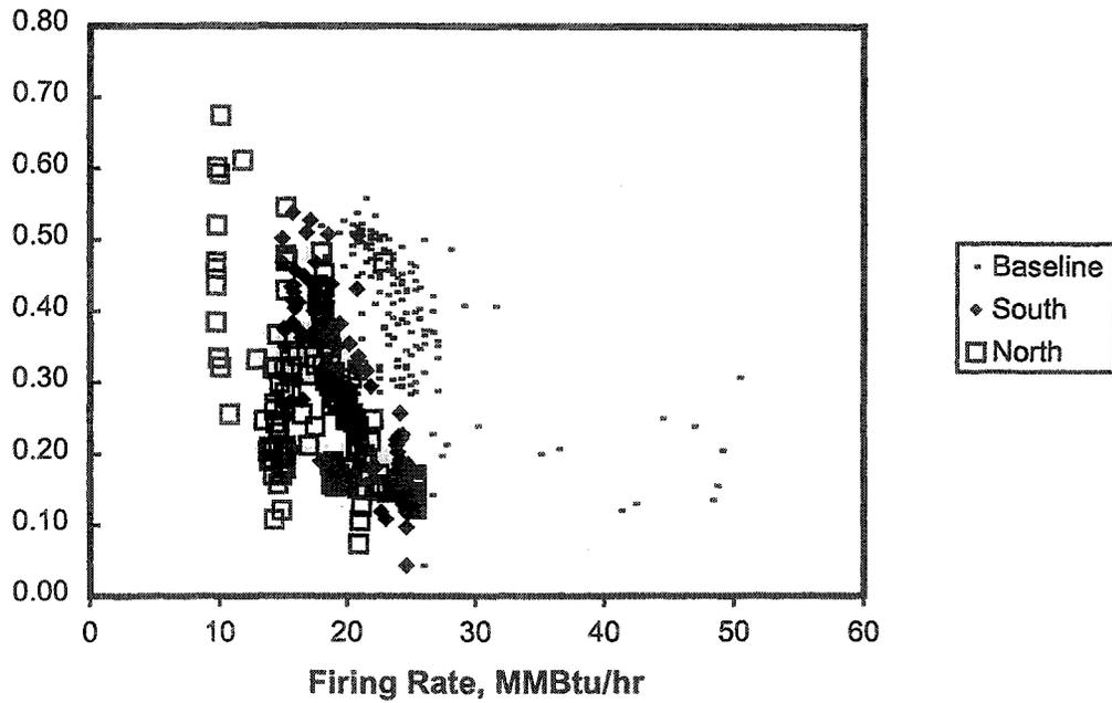
Figure 5. Furnace NOx as Function of Firing Rate for Oxy-Fuel Tests
