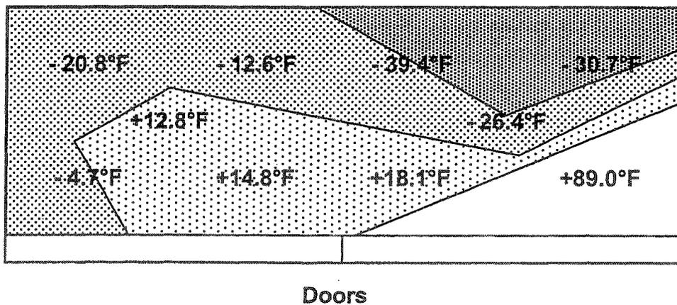
Figure 1. Deviation of Average Thermocouple Readings from Overall Average of 2332.2°F
