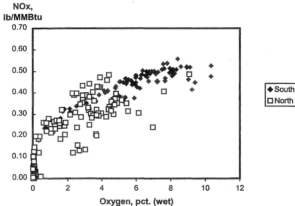
Figure 2. Furnace NO<sub>x</sub> as Function of Excess Oxygen Level for Baseline Tests
