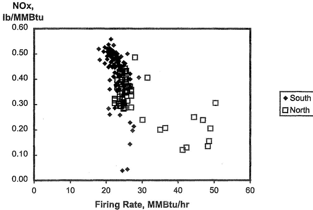
Figure 3. Furnace NOx as Function of Firing Rate for Baseline Tests
