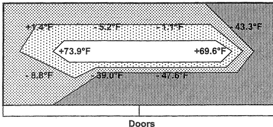
Figure 4. Deviation of Average Thermocouple Readings From Overall Average of 2275 F, with Burners Biased Toward Doors
