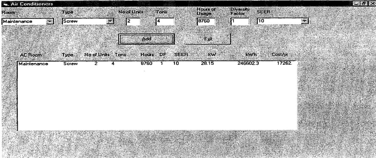
Figure 7. The Air Conditioners Interface Screen
