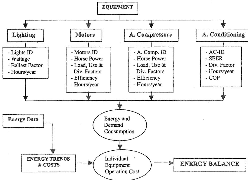
**Figure 2. The Interactive Energy Balance (IEB) Simplified Data Flow Diagram**
