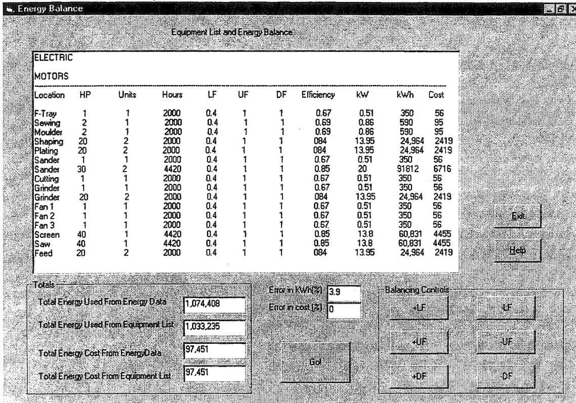
**Figure 8. The Equipment List and Energy Balance Chart. Also Shown Is The Balancing Options Screen, Which Includes The GO ! Button to Balance The Equipment Energy Consumption Against Electrical Energy Bills**
