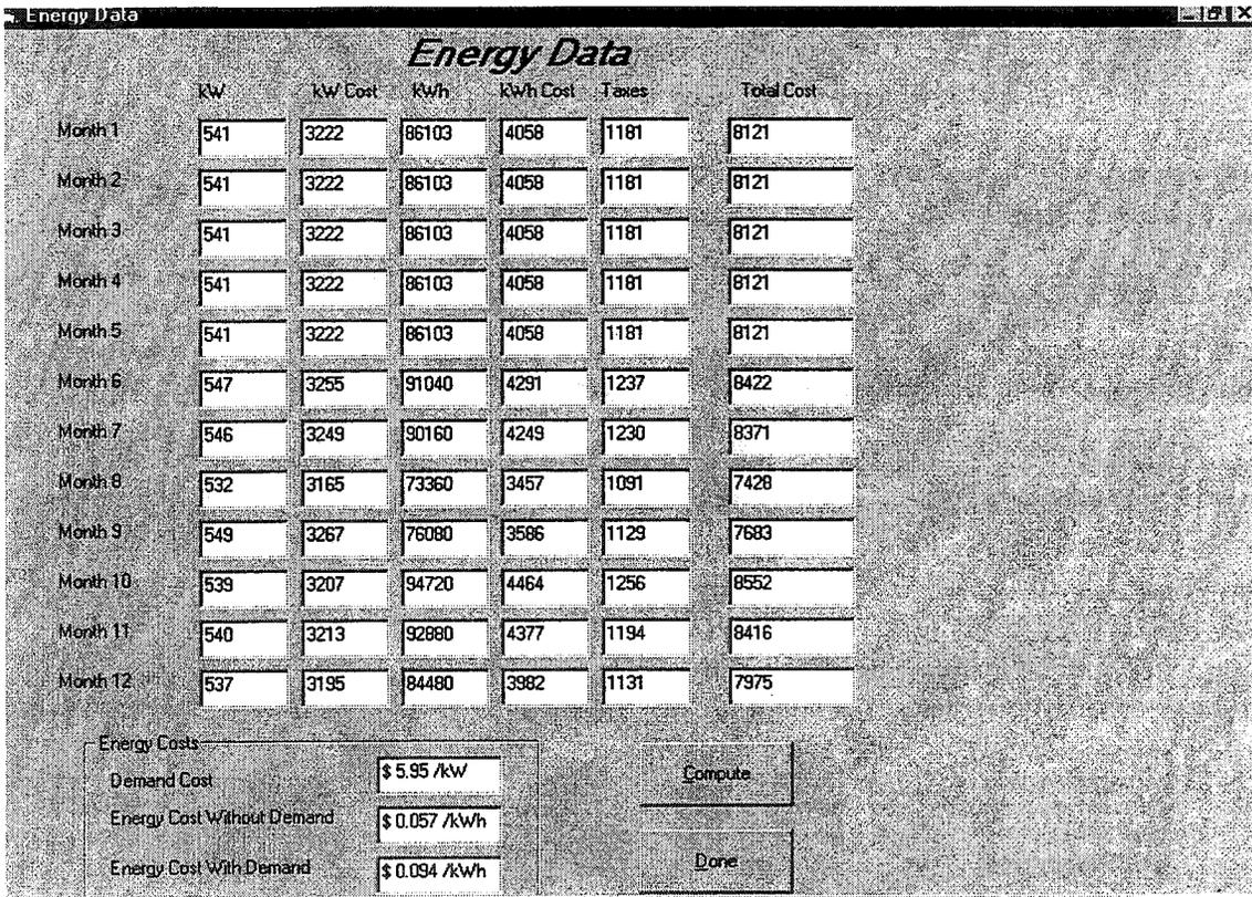
Figure 3. Energy Data screen where Historical Electrical Data Should Be Entered (data energy costs parameters are determined from these input data)
