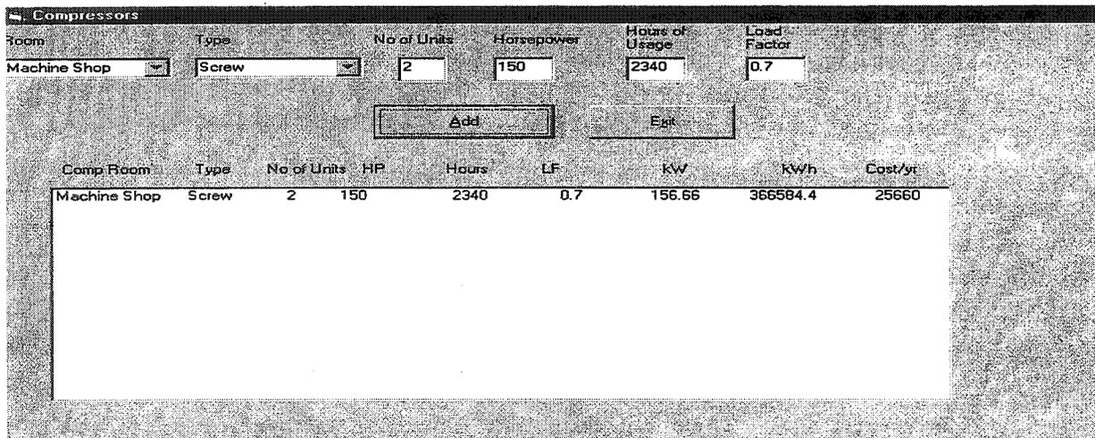
Figure 6. The Air Compressors Interface Screen
