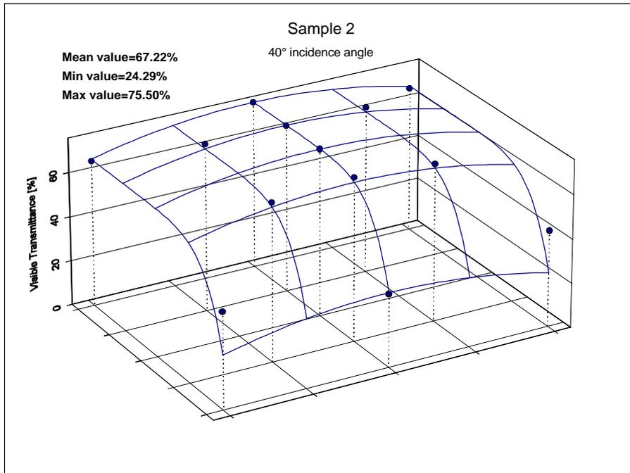
**Figure 6. Interpolation surface of S2 Light Transmittance Measurements at 40°**
