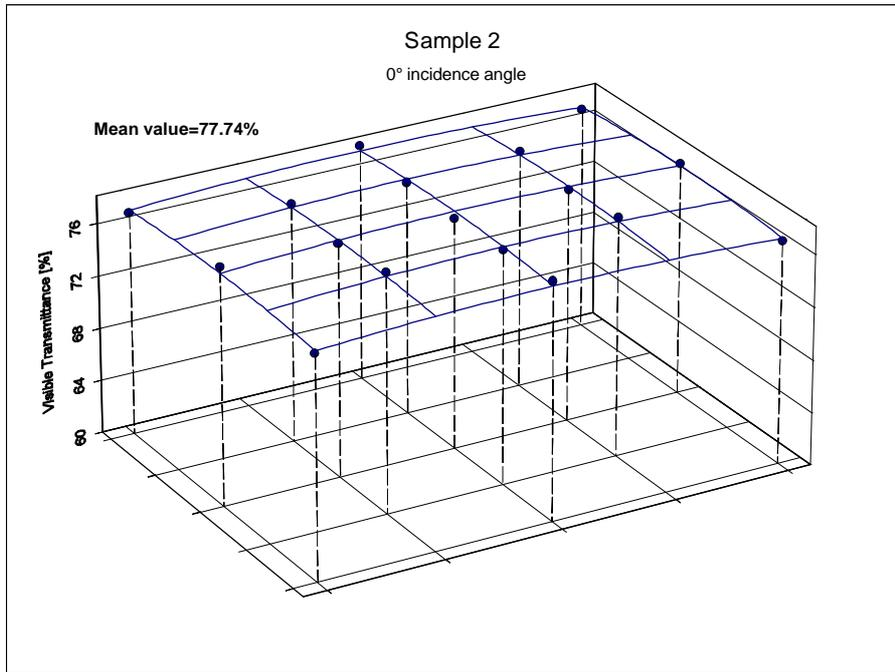
**Figure 4. Interpolation Surface of S2 Light Transmittance Measurements at 0°**
