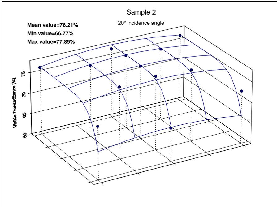
**Figure 5. Interpolation surface of S2 Light Transmittance Measurements at 20°**
