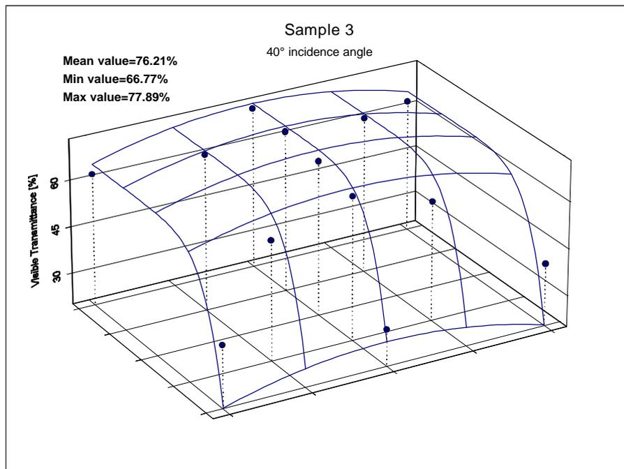
**Figure 8. Interpolation surface Light Transmittance Measurements of S3 at 40°**
