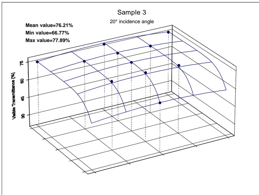
**Figure 7. Interpolation surface of S3 Light Transmittance Measurements at 20°**
