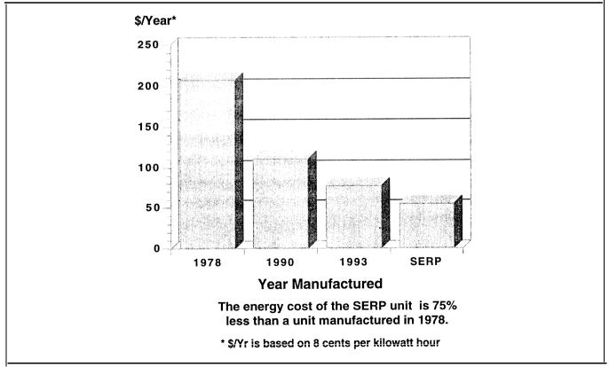
Figure 2. Annual Cost of Refrigerator Operation
