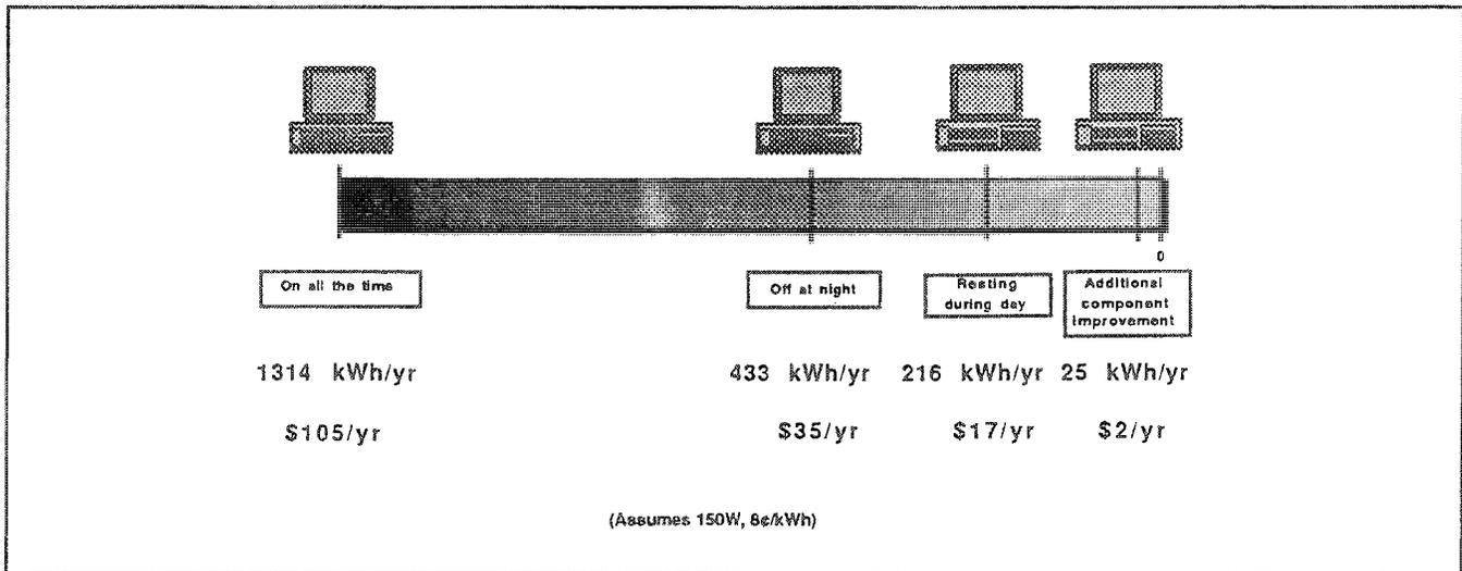
Figure 3. Electricity Consumption and Costs for Inactive Personal Computers
