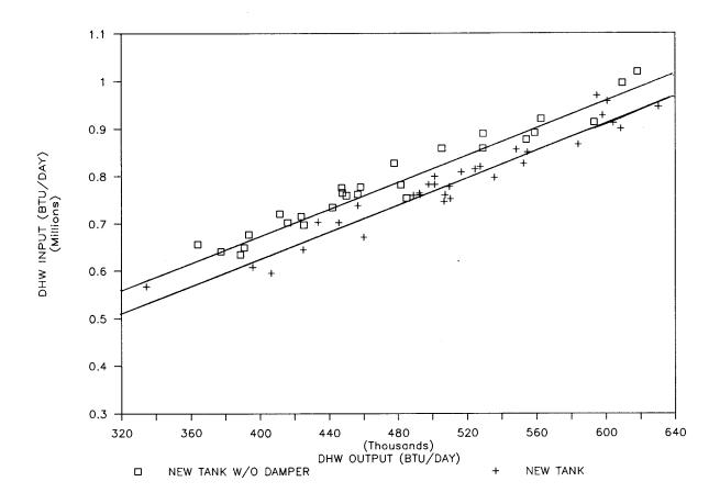
FIGURE 1. Performance of new tank water heater.
