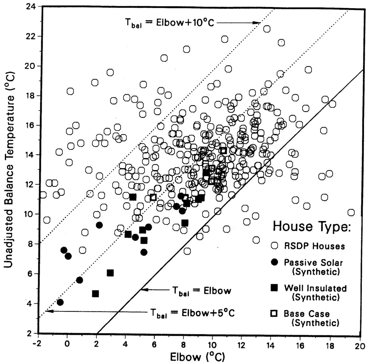
Figure 8. Elbows vs. Balance temperatures for real and synthetic data. The regression-derived balance temperatures lie several degrees above the elbow temperatures. This suggests that significant floating is already occurring in the homes below the balance temperature. Similar trends were seen in both the synthetic and real data.
