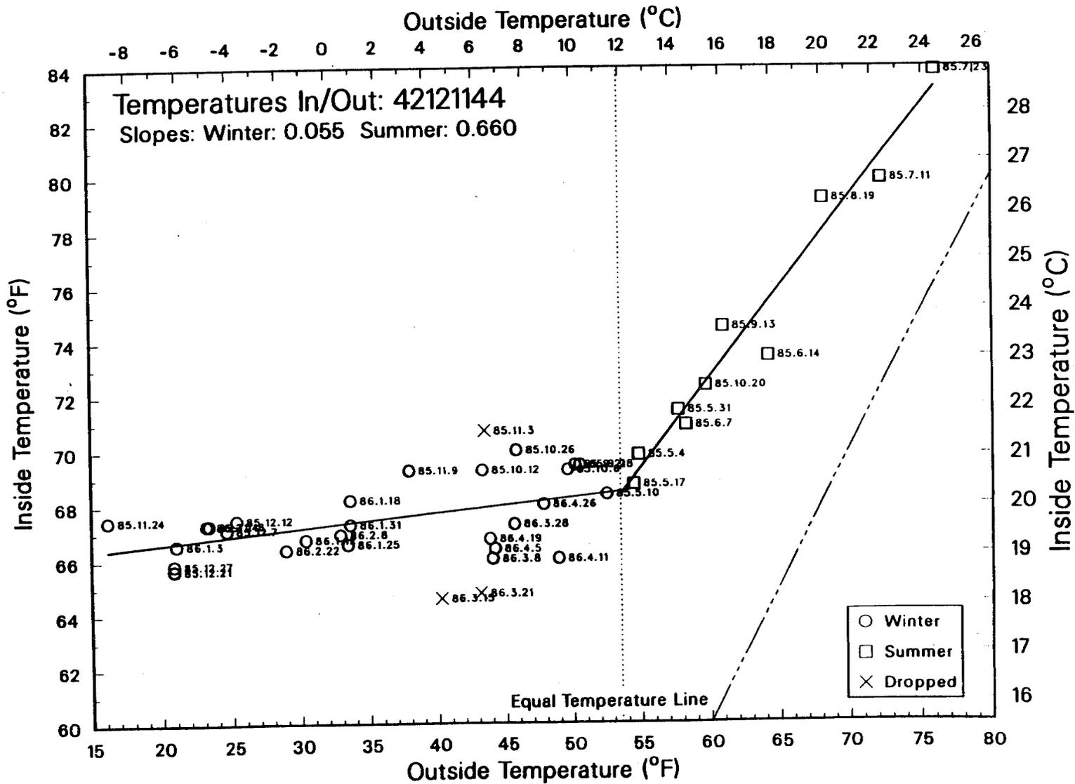
Figure 7. Scatterplot of outside-inside temperatures for a RSDP house. The scatterplot shows the Winter and Summer regression lines. The shallow slope of the Winter line suggests that the occupants maintain a relatively constant indoor temperature.
