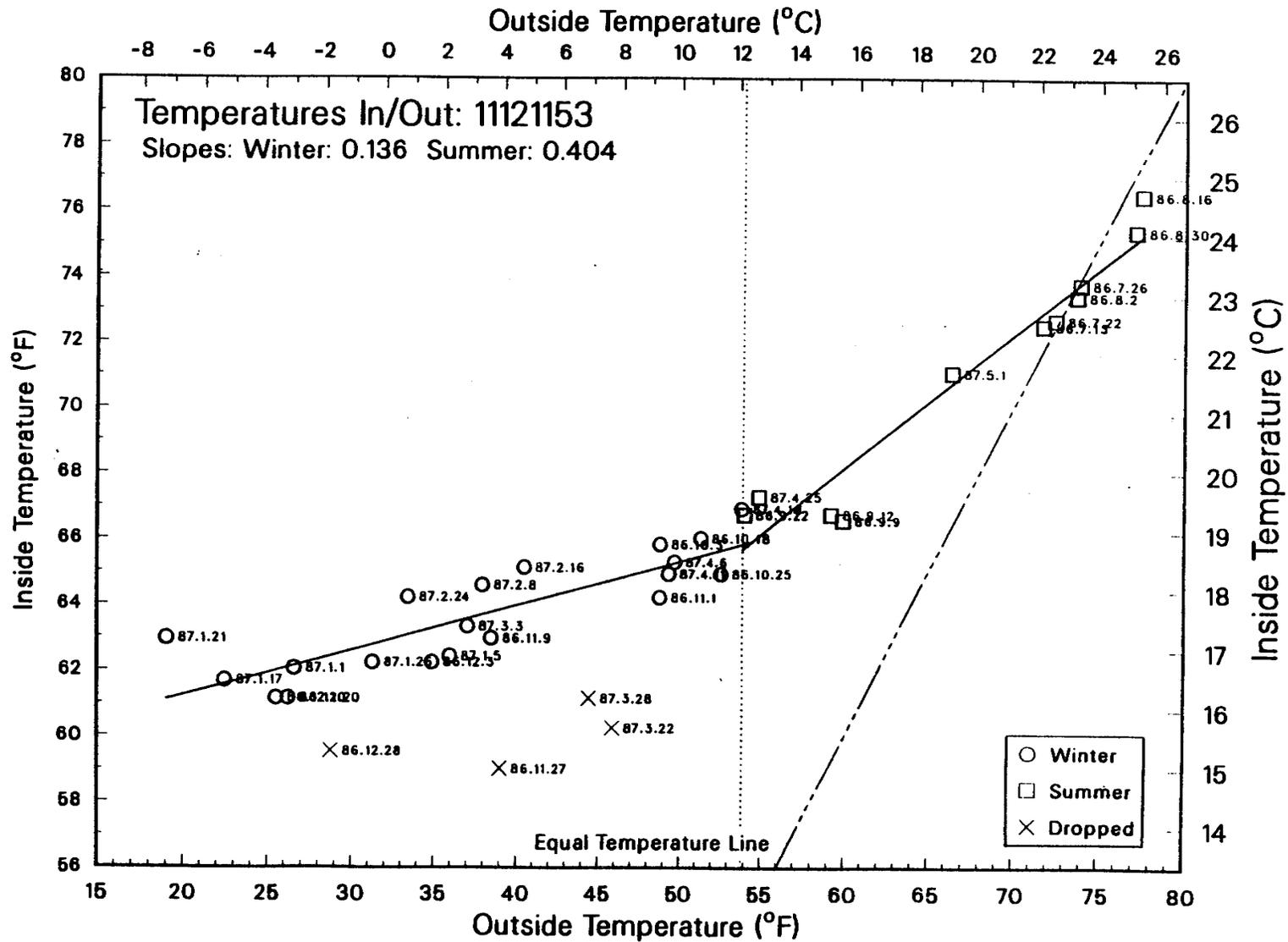
Figure 6. Scatterplot of outside-inside temperatures for a RSDP house. The scatterplot shows the Winter and Summer regression lines. Note the slope of the Winter line, suggesting that the occupants set back the thermostat.
