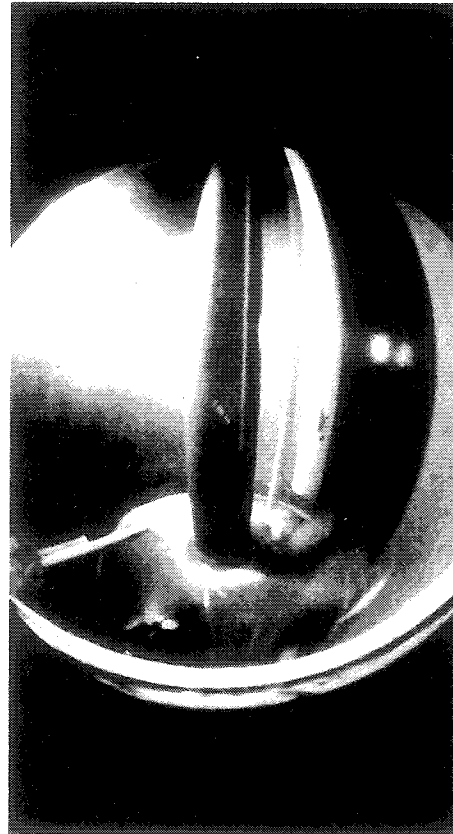
HEATER G-5 SOFTENED WATER 27,000 GAL THROUGHPUT 166 F OUTLET TEMP
