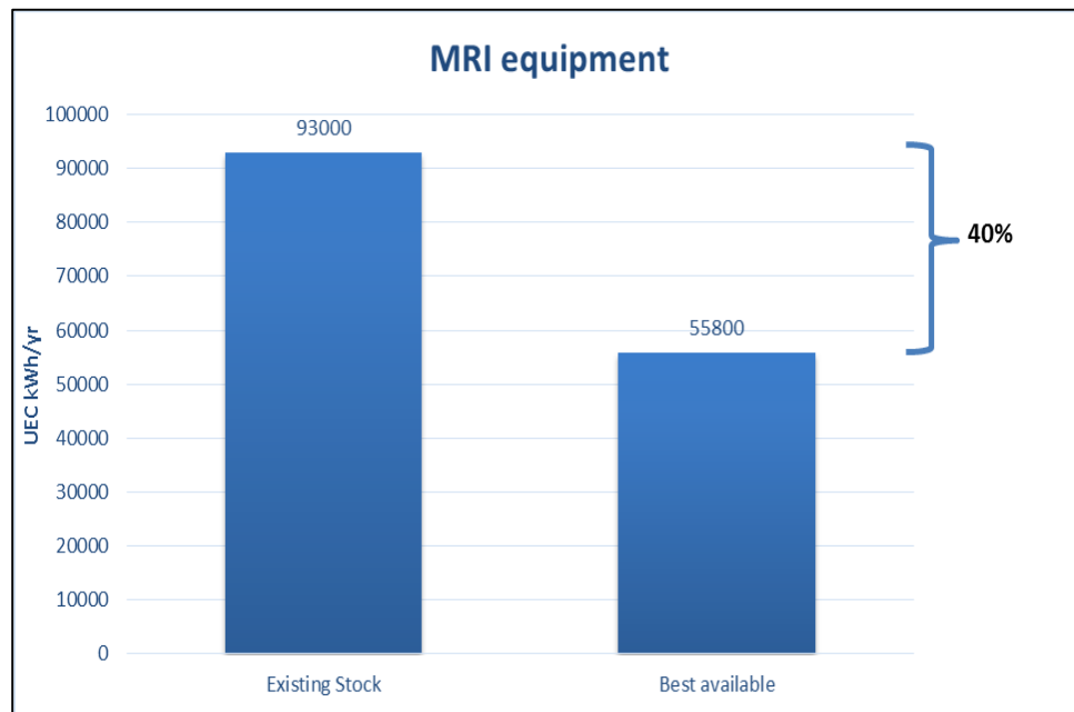
Figure 34: Energy Saving Potential
