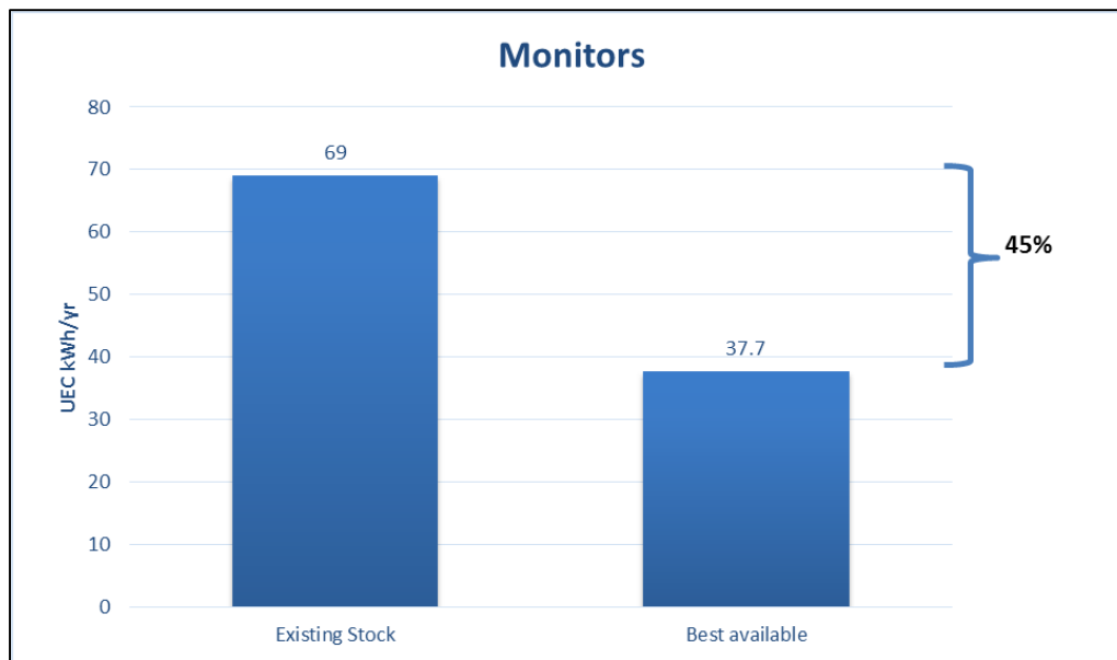
Figure 16: Energy Saving Potential
