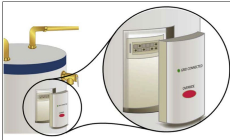
Figure 1. Port and communications module on a water heater.
